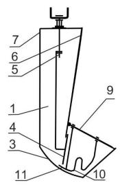
Fig. 7.10. Vertical section of the feeder for pigs
