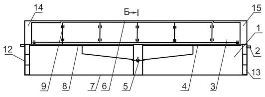
Fig. 7.9. Horizontal section of the feeder for pigs
