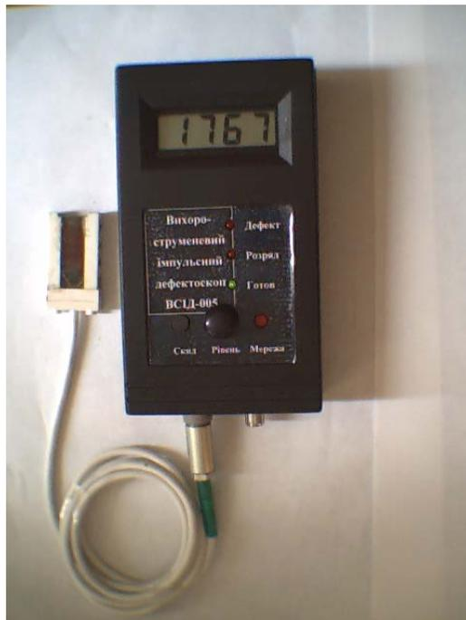
Fig. 2.1. Appearance advanced pulsed Eddy current flaw
