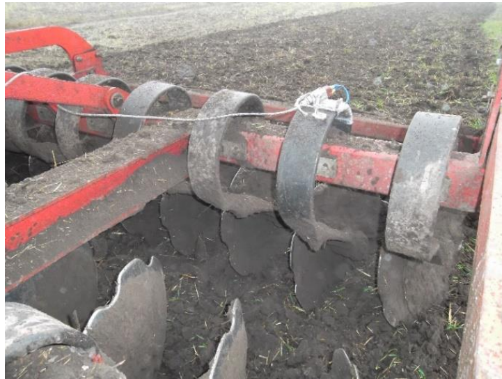
Fig. 14.2 The movement of the oscillating system “soil – disk – spring shank”.
