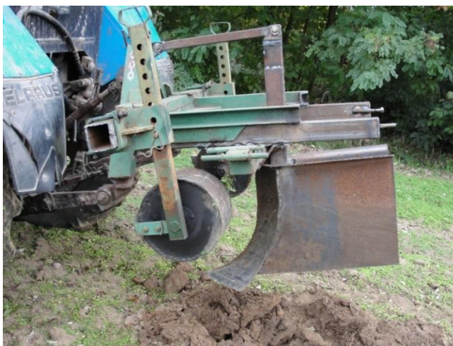
Figure 1.5. Prototype of the working body of the orchard planting machine during experimental research and testing.
